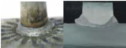
View and penetration shape of an optimized W-S stud welding
